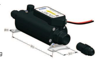
Within the body of the PX375-TC Boost Pump is contained the Bypass. This feature allows for fuel to flow around the positive displacement pump, whilst the pump is not running. The porting within the body has been computer optimised to ensure the best possible flow conditions.
