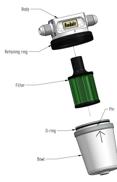
Remove safety wire from the black retaining ring.
