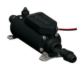
Within the body of the PX375-TC Boost Pump is contained the Bypass. This feature allows for fuel to flow around the positive displacement pump, whilst the pump is not running. The porting within the body has been computer optimised to ensure the best possible flow conditions.
