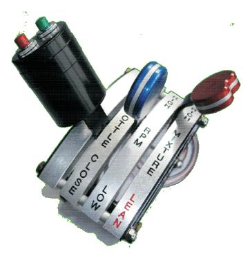
Each lever is guided by Teflon® pads at the top to give a feel that is both smooth and accurate. Along the base is a friction nut that can be used to lock all three levers, although this can be overridden with a gentle pressure.
