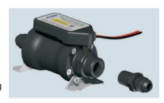
The Andair Brushless Fuel Pump motor is immersed within the fuel. This has 3 distinct advantages; the fuel can be used to cool the internals and the design ensures there will never be any leaks between the drive to the pump, furthermore, using advanced materials and machining techniques we can use the fuel to lubricate the internals giving us better performance.
